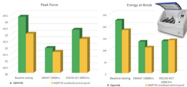
Fig. 7 – Bond strength retention following exposure to 1000 hours cyclic corrosion and SWAAT
